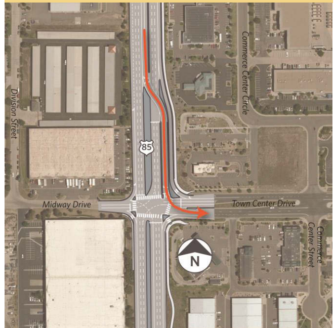
Figure 10. Town Center Drive Continuous Flow Intersection
