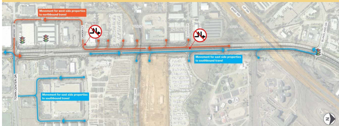
Figure 12. Town Center Drive Continuous Flow Intersection U-Turn Access
