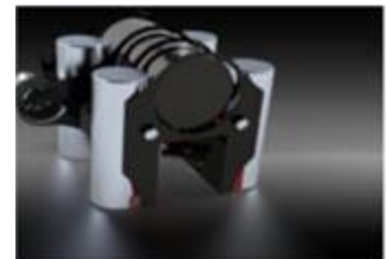
Figure 14: Solidworks design showing placement of buoyancy tanks
