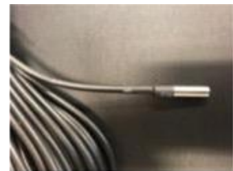
Figure 23: Temperature Sensor Photo Credit: N. Lees
