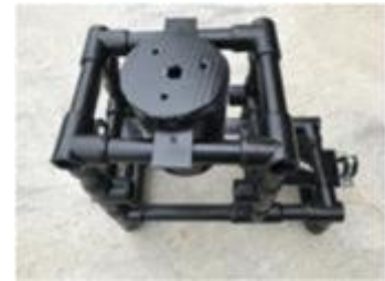
Figure 35: Grout Dispenser and Trout fry basket Photo Credit: N. Lees
