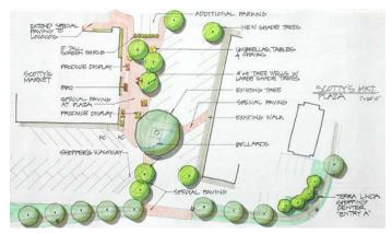
Angled parking with one driveway is more convenient but causes a net loss of four parking stalls. Ninety degree parking and one driveway result in no net loss of parking. Once the parking realignment is achieved, important connections need to be made to the Terra Linda Recreation Center and to the new walkways on Freitas Parkway.
