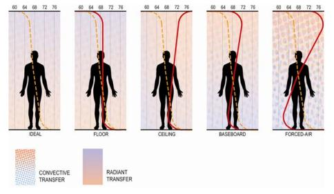
Figure 3: Temperature Profiles
