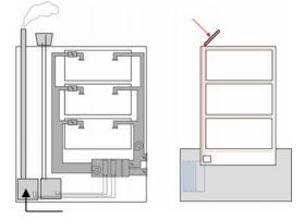
Figure 6: Volumetric Impact of Air and Water Systems
