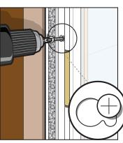
**5F** Close the door and push it tight against **5G** Cut rail extender weatherstripping door frame. Pre-drill holes and install mounting frame screws on the outer side of hinge rail. Do not over tighten screws.
