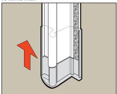
**7D** Align the edge of the drip cap with the outside edge of the latch rail. Verify the door closes freely without hitting the latch rail.
