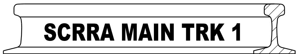
TYPICAL MARKING ON WEB OF RAIL
