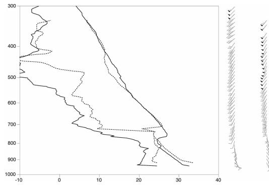
FIG. 5. Skew *T*-log*p* diagram of the NCAR M-CLASS soundings. Profiles are at 1830 UTC (solid lines, and set of wind barbs on left), and 2030 UTC (dashed lines, and set of wind barbs on right). Location of the 1830 and 2030 UTC launch sites are shown in Fig. 4.
