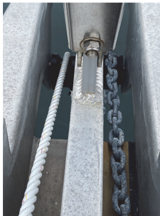
Long snubber run on 2nd bow roller
