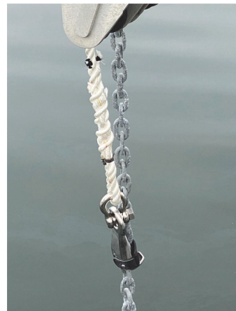
Mantus chain hook attached-this should be let out 20-30'
