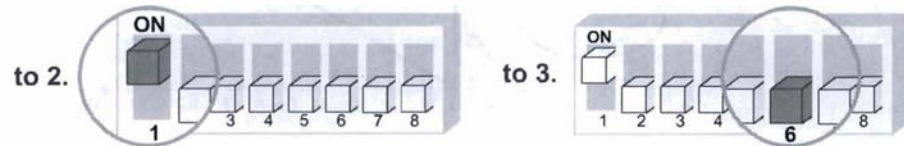
Fig. 9: Setting DIP switches
