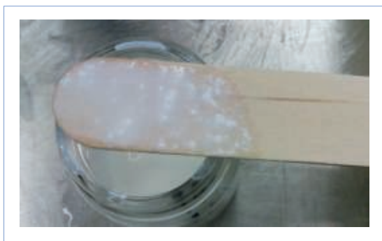
Figure 4 —Grit formed when hardener was mixed with AEH.
