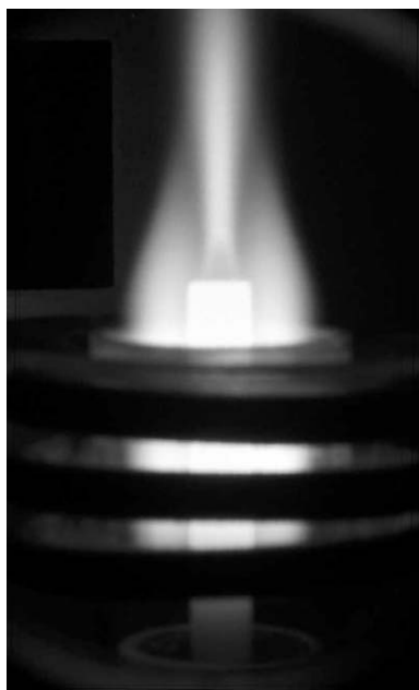
Fig. 12 Image of the ICP with sample probe insertion showing the inverted cone of Ba emission at the tip of the sample probe. Sample probe diameter was 4.6 mm. Opening of the probe was 1.7 mm. Probe insertion position was 6 mm HALC. Carrier Ar gas flow rate was 0.42 \text{ L min}^{-1} .
