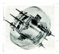
The output or plate end of the double pentode. The thorough shielding is accomplished by the metal ribbon cylinder
