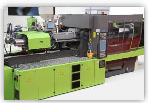
The moulds used in these machines are made out of metal and cost roughly V\$50,000 to produce. The moulds have finite lives, eventually losing their precise shape. The bricks have to be manufactured to a very precise tolerance, otherwise they will not fit together properly. Prybloxx minimises the numbers of moulds required by aiming for long production runs of each given part.
