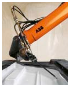
Figure 8: Thanks to its long injection lance, the KraussMaffei MK 2.0-2K-S-L spray mixing head is also good at making undercuts in complex parts. (Photo: KraussMaffei)
