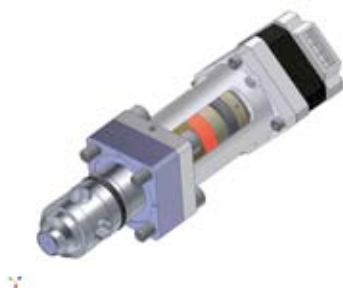
Figure 3: Thanks to a new nozzle concept patented by KraussMaffei, an electric motor only has to work against very low pressure moments. Thus, the needle can be moved effectively and quickly. Consequently, component pressure under varying dispensing rates can be regulated quickly and kept stable. (Graphic: KraussMaffei)
