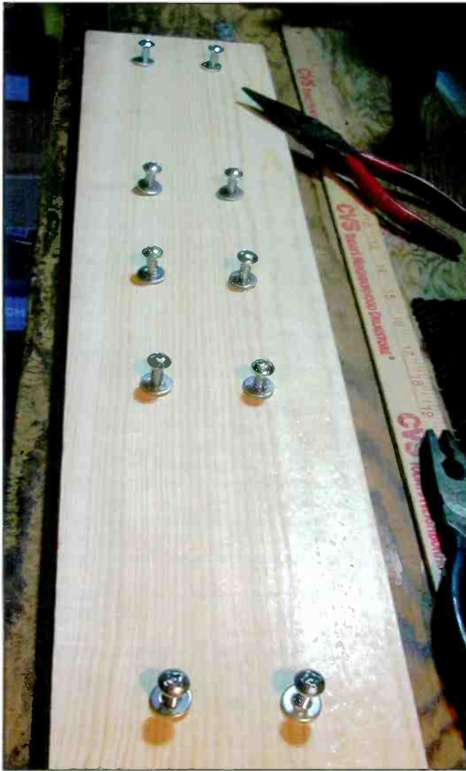
Photo G: After sketching where screws and washers will go to affix the antenna elements and phasing lines, they're loosely mounted on the wood DTV antenna board. The accompanying drawing shows where they are positioned.
