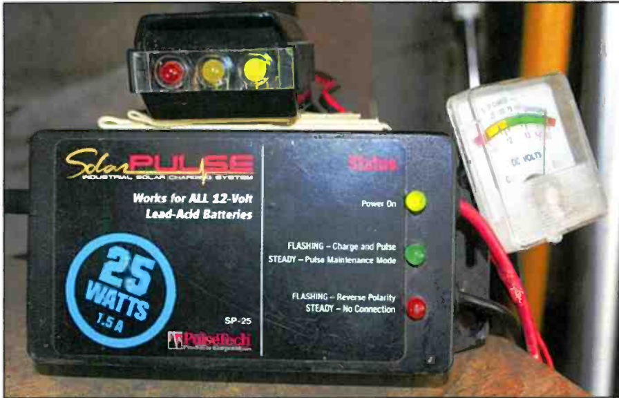
This is a solar panel pulse charger status indicator, with added voltage monitors
