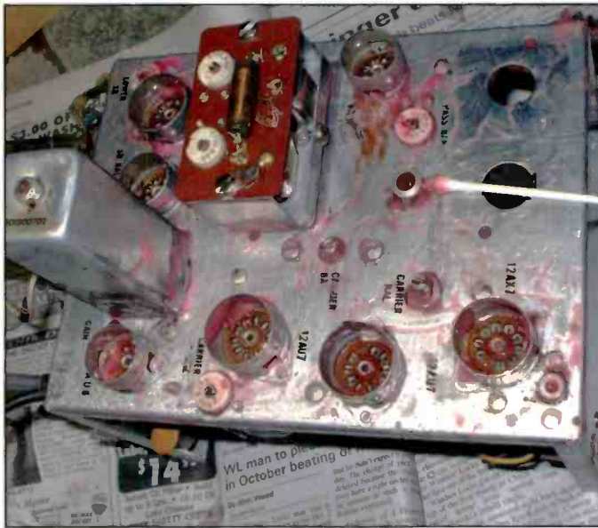
Photo G: Again, naval jelly was carefully applied to the SSB generator subchassis. This product can cause more problems than it cures if allowed to come in contact with components or sockets.
