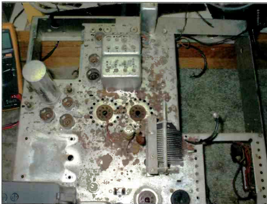
Photo E: Alas, once the chassis was stripped of what was reasonably easy to remove, the extent of the damage was easier to see.
