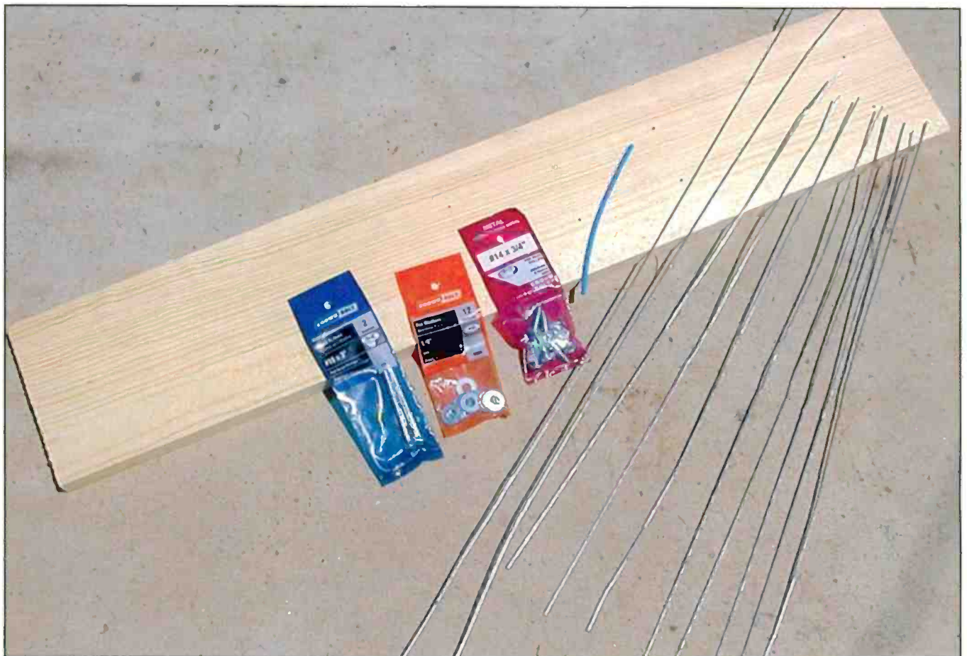
Photo E: Simple hardware, coat hangers, a piece of wood and a handful of other parts are used to construct this simple-but-effective DTV antenna.
