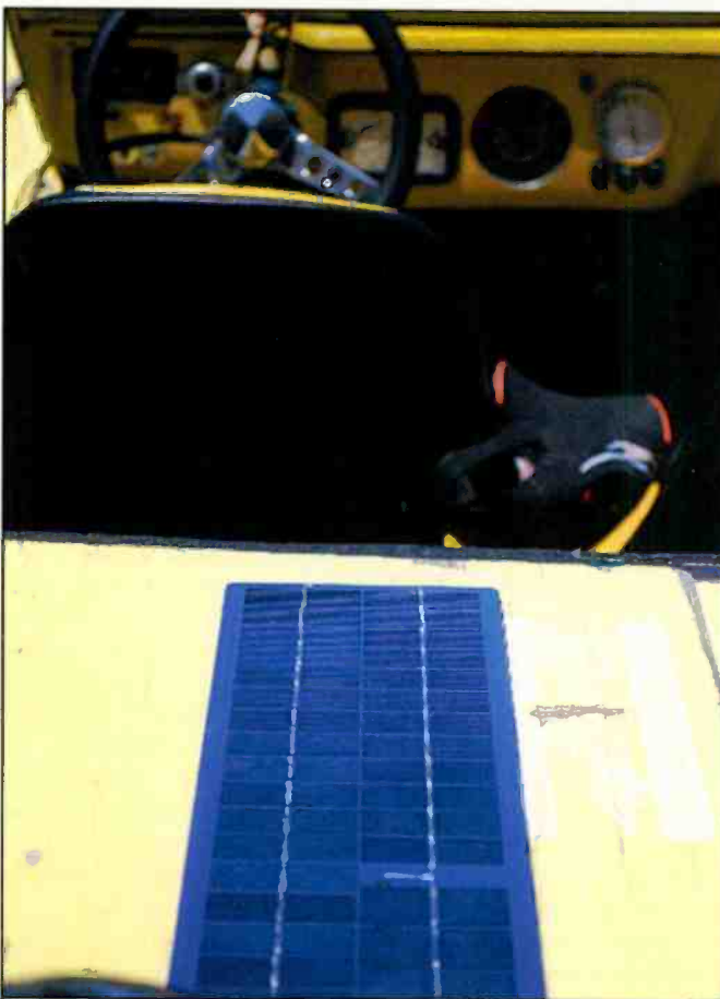
A small solar panel is used with the pulse charger in Gordo's dune buggy.
