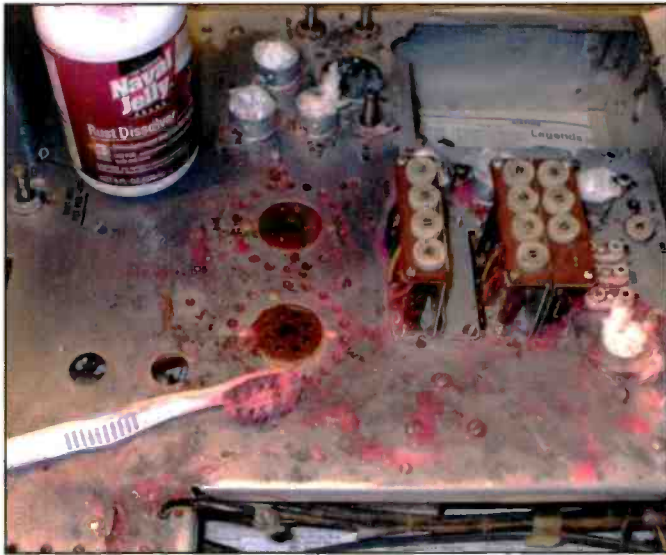
Photo F: Naval jelly, which uses phosphoric acid as an active ingredient, was applied with a toothbrush over the rusted areas.
