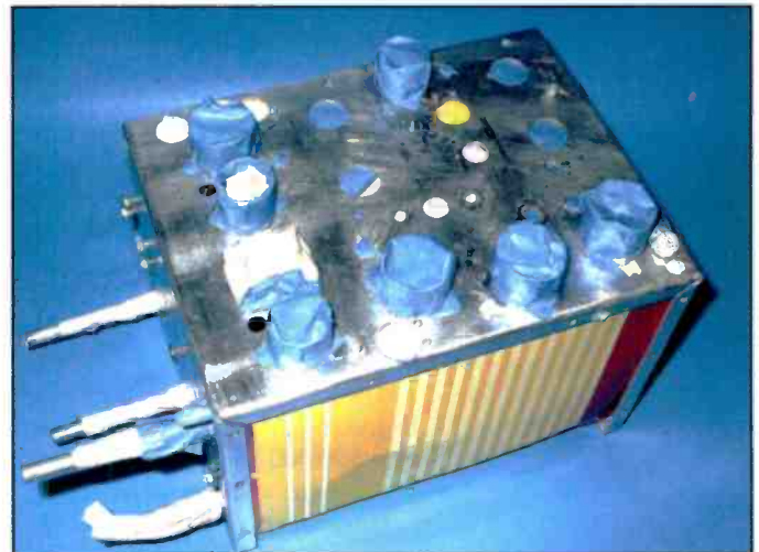
Photo I: The SSB generator is now free of rust, but the chassis plating was ruined.
