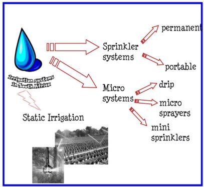
The above diagram gives and overview of the different types of irrigation systems.
