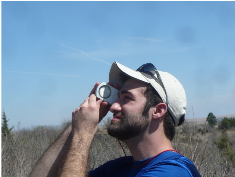
Figure 3. The clinometer measures the angle between the object being viewed and level.
