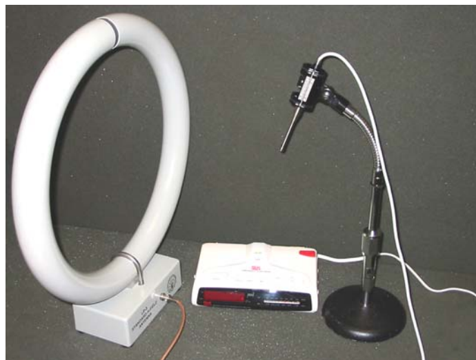
Figure 20 - Acoustic testing of Sima table radio with Bruel & Kjaer instrumentation microphone inside acoustic box of 1-ft. thick closed-cell foam. Magnetic field loop antenna also shown.
