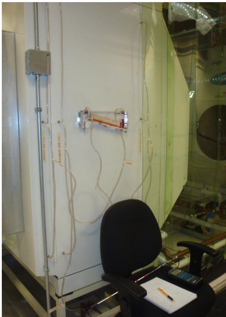
Figure 17. Pressure differential measurement setup in NSIDC on CU4.
