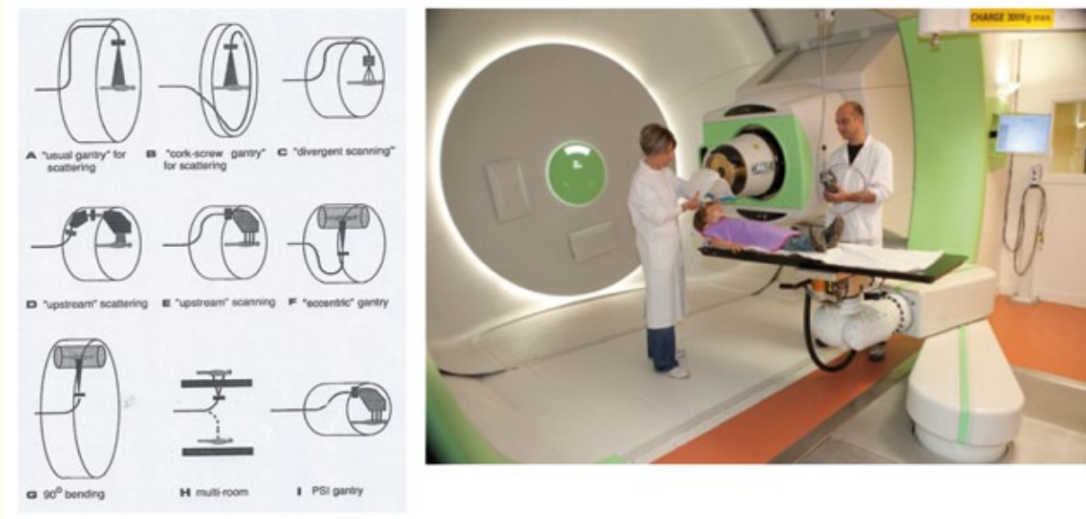
Figure 4.2. (a) Different kinds of gantry (Pedroni et al. ). (b) Gantry (patient enclosure) at Institut Curie.
