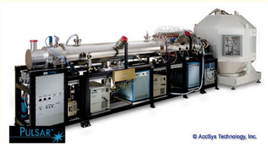
Figure 2.7. A 7 MeV Proton linac for PET isotope production from ACCSys. [ http://www.accsys.com ]
