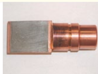
Figure 2.14. Example of a multipurpose internal slanted solid target with extremely low angle suitable for production of e.g. ^{67}\text{Ga} , ^{111}\text{In} or ^{201}\text{Tl} (Nuclear Physics Institute AS CR, v.v.i., Řež) [Leb05].
