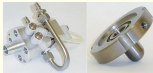
Figure 2.15. Liquid target (left) and its niobium chamber (right) for production of ^{18}\text{F} that can be also operated as solution target for production of ^{68}\text{Ga} or ^{86}\text{Y} (Nuclear Physics Institute AS CR, v.v.i., Řež).
