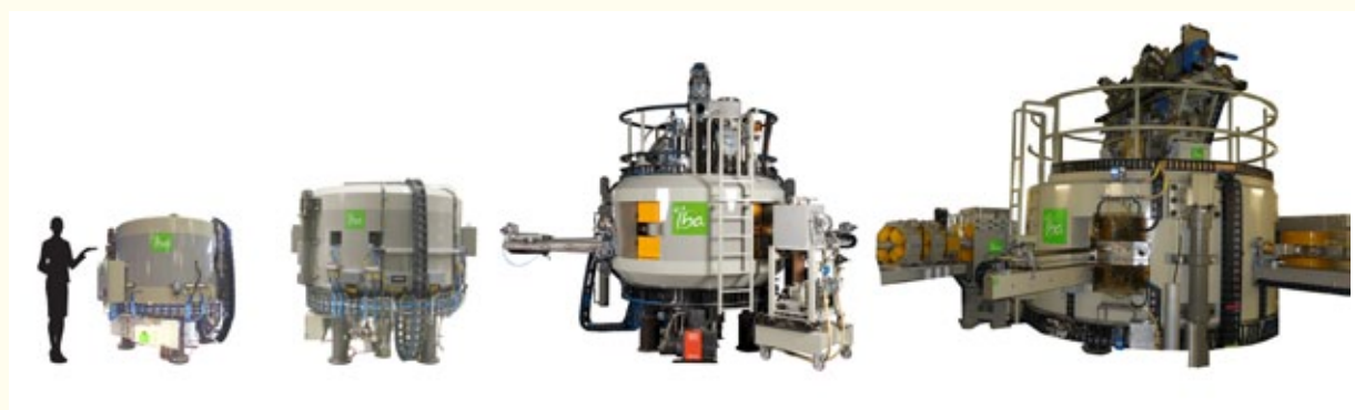
Figure 2.5. Typical sizes of IBA cyclotrons providing proton energies of 11, 18, 30 and 70 MeV from left to right.
