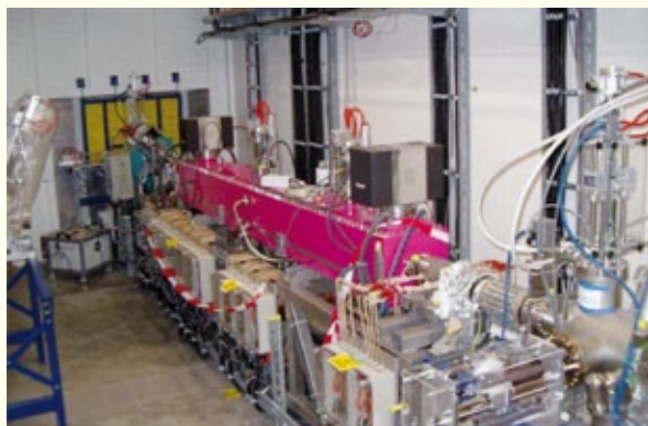
Figure 2.8. View of the 7 A×MeV linac at the cancer therapy centre HIT, Heidelberg, Germany.
