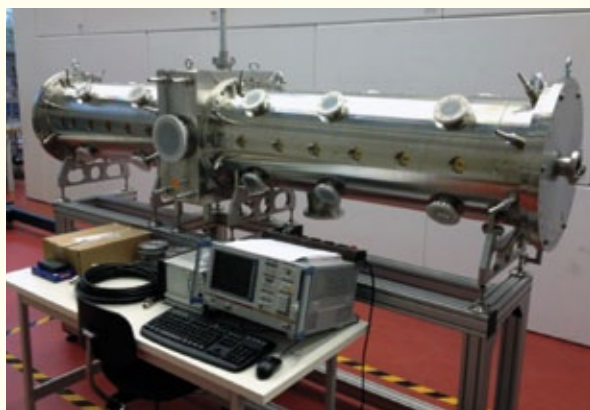
Figure 2.9. 325 MHz prototype CH – cavity accelerating from 11.7 MeV to 24.3 MeV within a tank length of 2.9 m.
