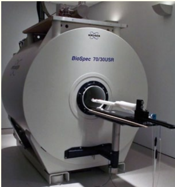
Figure 5. A typical MR system for small animals (Taken from: http://www.weill.cornell.edu/research/cbic/facilities/mri_7tesla.html )
