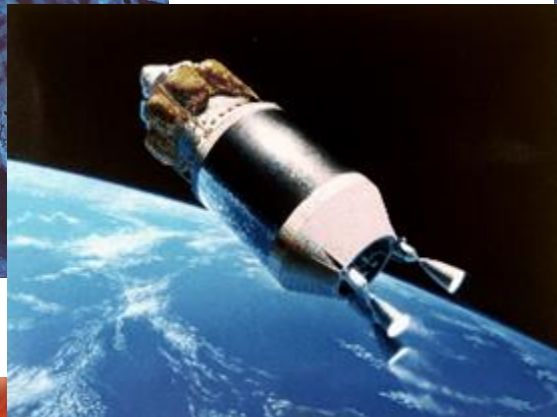
Expendable TLI Stage for First Lunar Outpost Mission using Clustered 25 klb f Engines -- "Fast Track Study" (1992)
