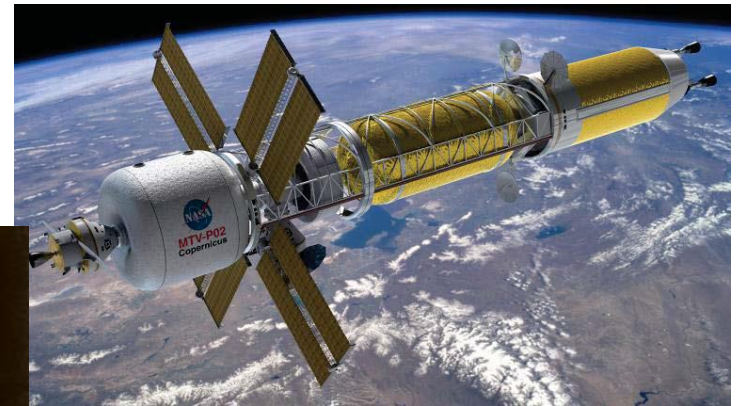
Zero-Gravity Crewed MTV uses 3 - 25 klb f NTR Engines & PVA Auxiliary Power -- Mars (2009)
