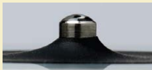
Droplet "flattens out" on unconditioned pedestal
