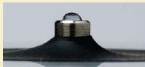
Droplet "beads up" on properly conditioned pedestal
