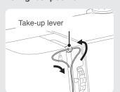
Turn the pulley to bring the take-up lever to its lowest position and pass the thread through the thread guide.
