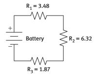
The control circuit for the heater circuit (shown above) is not working properly. George needs to troubleshoot to find where the problem is. The heater elements are represented by  $R_1$ ,  $R_2$ , and  $R_3$ . If  $R_1 = 3.48$  ohms,  $R_2 = 6.32$  ohms, and  $R_3 = 1.87$  ohms, George must figure out how much total resistance (measured in ohms) the circuit has.
