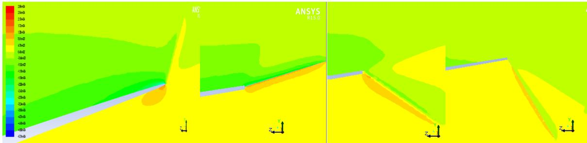
Figure 10: Pressure contours of four winglets at  $\alpha = 2.5^\circ$
