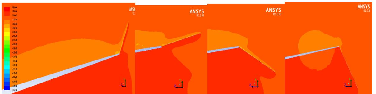
Figure 13: Pressure contours of four winglets at  $\alpha = 10^\circ$
