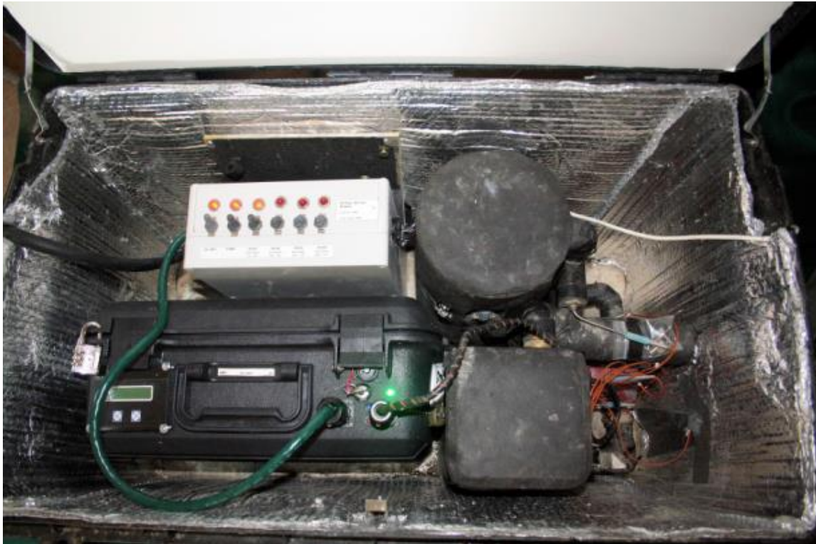
Figure 9: The TRT Test Unit used at the experimental test site.
