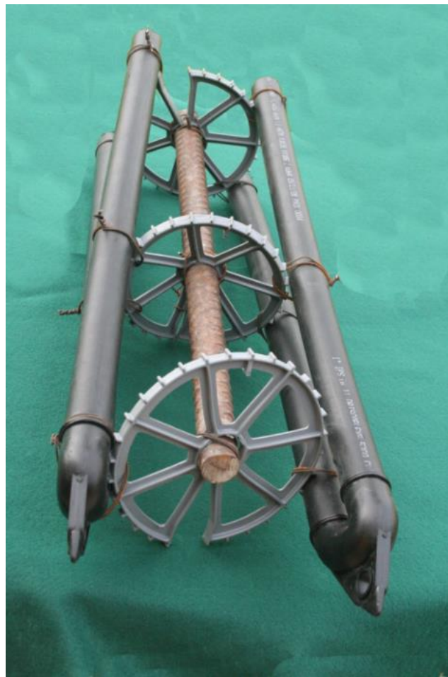
Figure 6: The loops used in the experimental piles from the Berkel test site.
