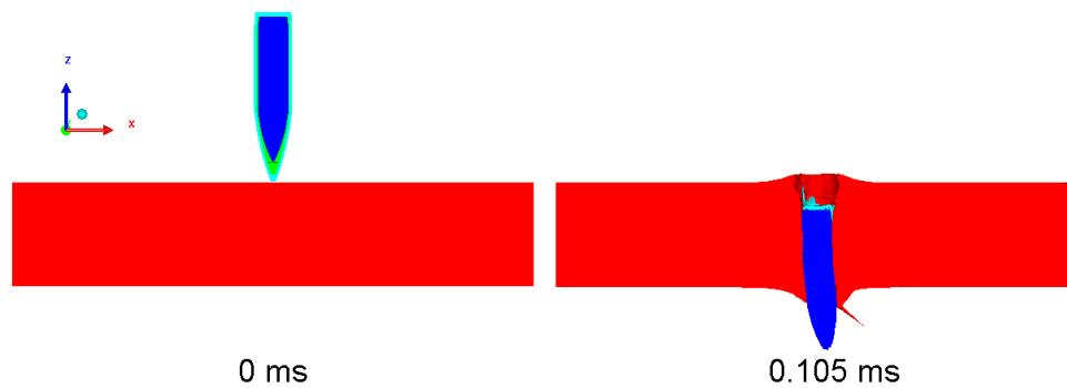
Figure 4.8: Simulation Result of the 20 mm Plate Impacted by the Bullet at 0^\circ
