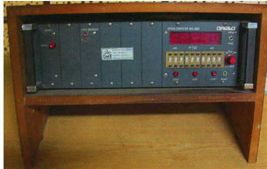
Figure 3.3: Speed Measurement Device
