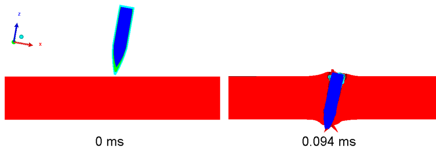
Figure 4.13: Simulation Result of the 20 mm Plate Impacted by the Bullet at 10^\circ
