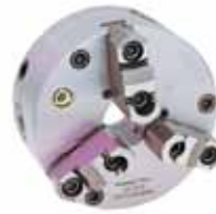
3565 3 Jaw Scroll Chucks. Two-Piece Hard Reversible Jaws, Dia. 5" to 25" Code No. 7-866-....
