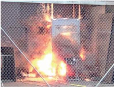
Photos of JNES High Energy Arc Fault (480V) Test 1 (left) and Test 2 (right)
