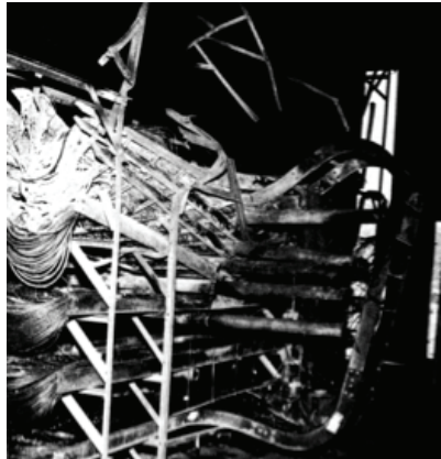
1977 Sandia National Laboratory full scale test with RG 1.75 separation criteria and IEEE-383 qualified cable – Before (left) and After (right)
