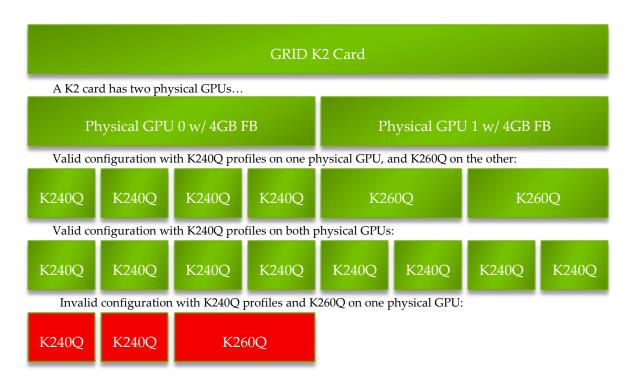
Figure 2-3. Example of a vGPU Configurations on GRID K2
