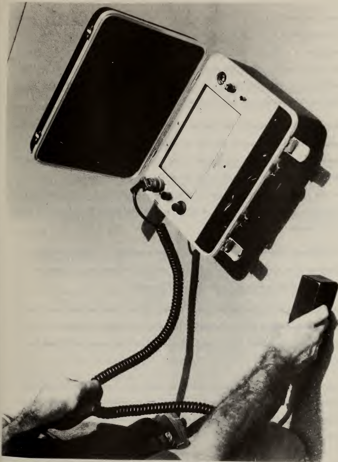
Figure 8. Cover meter used to detect steel reinforcement
