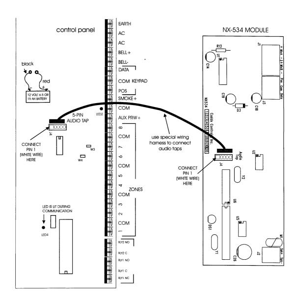
Check the correct position of PIN1 of the AUDIO TAP in the installation manual of the corresponding panel.
