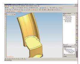
Abstraction commands are provided in the FEM for removal of design artifacts such as sliver faces, small edges and isthmus conditions. It does not remove the actual design features but rather allows for
