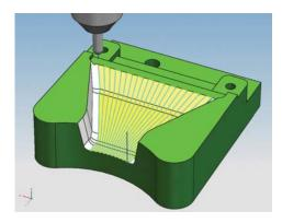
Variable-axis milling and profiling – NX supports both fixed and multi-axis milling functions on any NX part surfaces.
