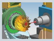
NX Mach 3 – Advanced 5 Axis Machining has the capability to take on any milling task within NX.
