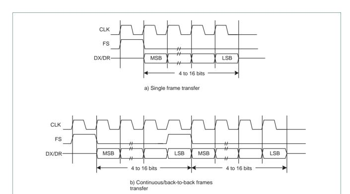
Fig 42. Texas Instruments synchronous serial frame format: a) single and b) continuous/back-to-back two frames transfer
