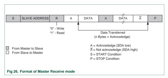
After a repeated START condition, I<sup>2</sup>C may switch to the master transmitter mode.
