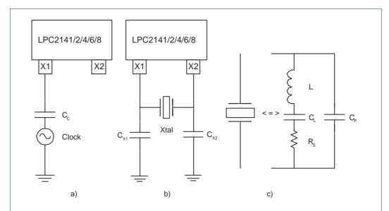
Fig 6. Oscillator modes and models: a) slave mode of operation, b) oscillation mode of operation, c) external crystal model used for  $C_{X1}/X_2$  evaluation
