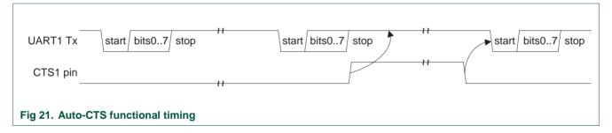
While starting transmission of the initial character the CTS1 signal is asserted. Transmission will stall as soon as the pending transmission has completed. The UART will continue transmitting a 1 bit as long as CTS1 is deasserted (high). As soon as CTS1 gets deasserted transmission resumes and a start bit is sent followed by the data bits of the next character.
