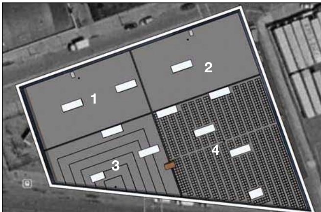
The rooftop was divided into four quadrants to study three different blue roof technologies in comparison to a control quadrant.
