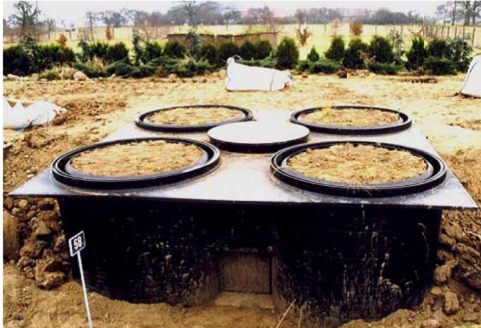
Figure 1.1: Polyethylene (PE-HD) lysimeter station with four lysimeters in a clover leaf arrangement with an entering hatch (center position) during the installation process. Source: Meissner et al. (2004).
