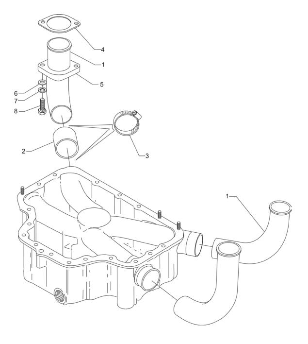
Intake Pipes and Attaching Parts Figure 12
