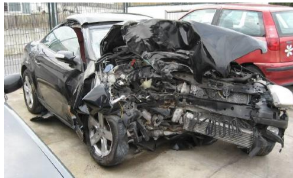
Fig. 6 – Damage to the Mercedes vehicle.
