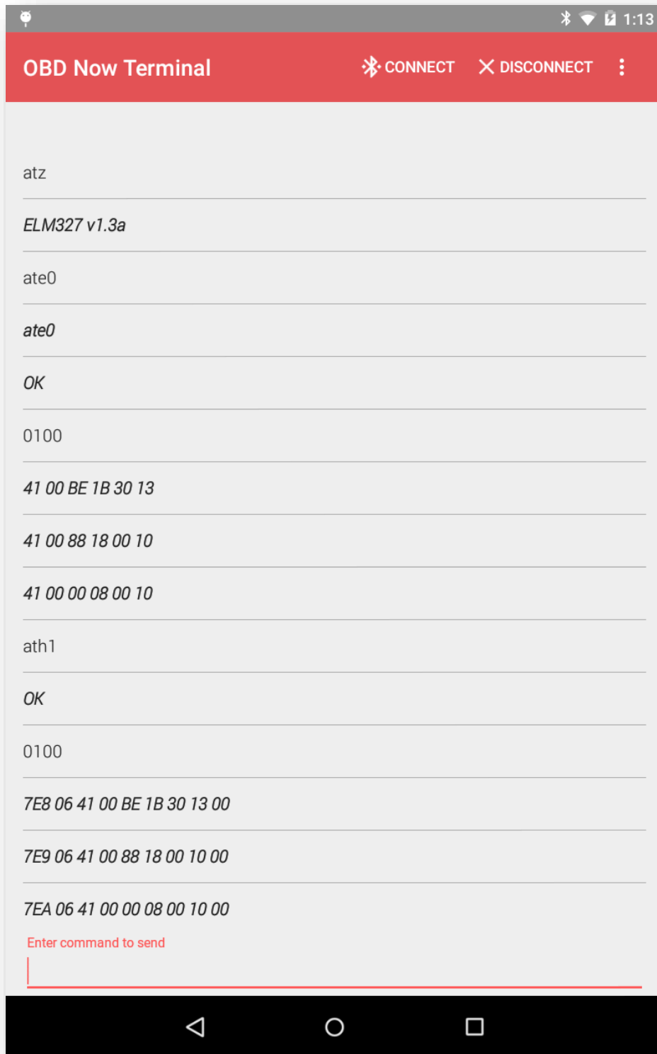
Figure 4 - 3 ECUs responding with Headers off and then on.
