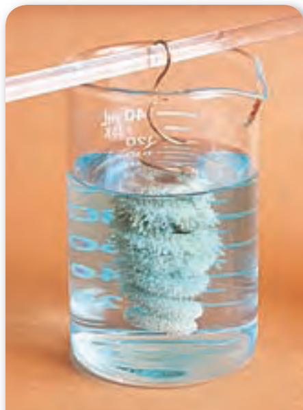
■ Figure 3.13 When a copper wire is placed in the solution of silver nitrate in the beaker, a chemical reaction occurs in which silver replaces copper in the wire and an aqua-colored copper nitrate solution forms.
