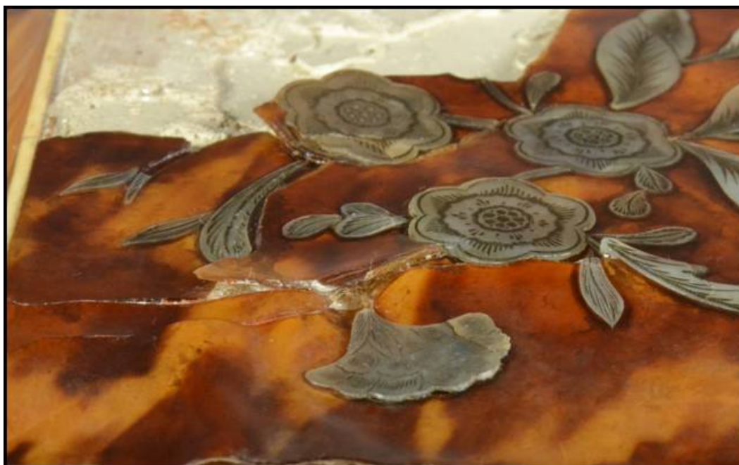
Figs. 8, 9. Sewing box top panel, details of cracking, splitting and dimension change (Photographs by Lori Trusheim)
