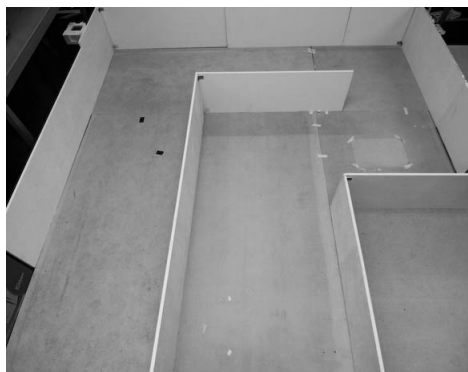
Figure 6.7: Photograph of maze setup. The beginning is in the bottom left-hand corner and the finish is in the lower middle part.
