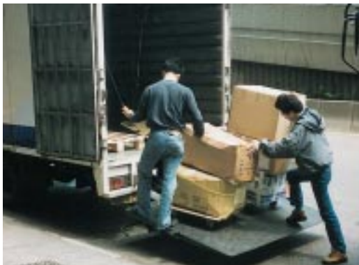
If a tailgate is used without a guard, trolleys can move suddenly.
