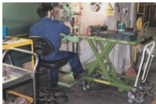
Use a trolley equipped with a scissor-lift and arrange the related works at the same work level.
