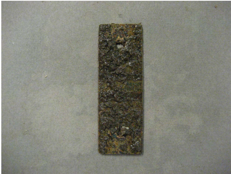
Figure 4-2: 90/10 Cu/Ni (CDA706) coupon, photographed 06/17/15.
