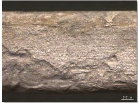
Figure 4-55: Z alloy screen at 50X magnification after cleaning.
