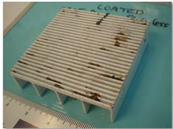
Figure 4-24: Coating damage to coated 2205 Duplex stainless steel wedge wire sample.
