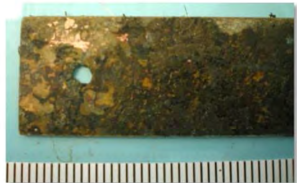
Figure 4-30: Detail view of 90-10 Cu-Ni 1-inch by 3-inch coupon with weld.
