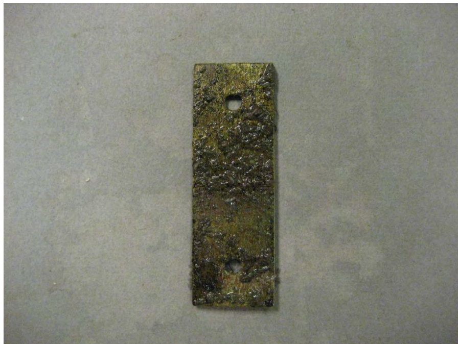
Figure 4-10: 70/30 Cu/Ni (CDA715) coupon, photographed 06/17/15.
