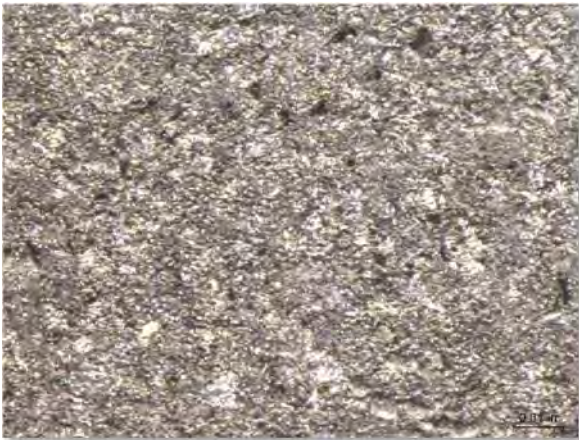
Figure 4-56: Z alloy plate at 50X magnification after cleaning.
