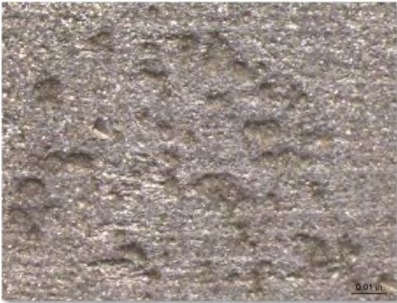
Figure 4-54: Z alloy coupon at 50X magnification after cleaning.
