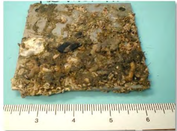
Figure 4-20: Marine life attached to uncoated 2205 Duplex stainless steel flat plate.
