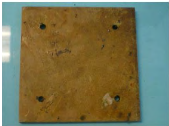
Figure 4-37: Minimal corrosion was observed on the Z alloy flat plate.
