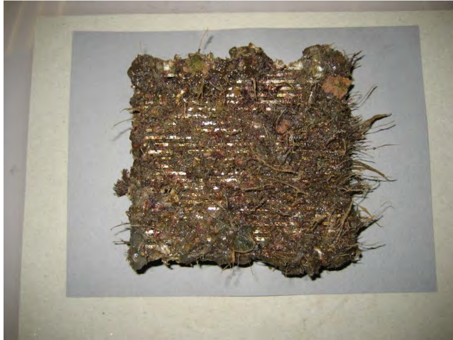
Figure 4-7: 2205 stainless steel Wedgewire sample, photographed 06/17/15.
