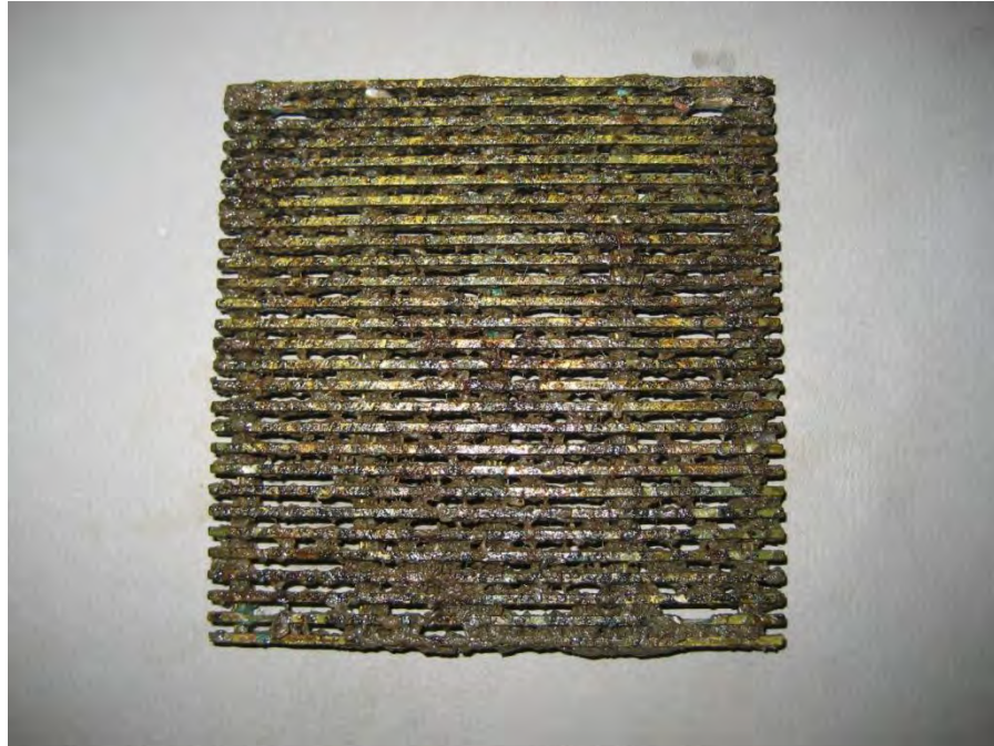
Figure 4-9: 70/30 Cu/Ni (CDA715) Wedgewire sample, photographed 06/17/15.
