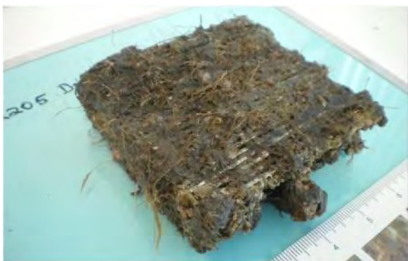
Figure 4-21: Marine life attached to uncoated 2205 Duplex stainless steel wedge wire screen.
