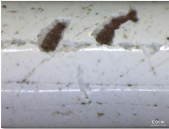
Figure 4-46: 2205 Duplex SS wedge wire screen surface exposed at an area of coating
