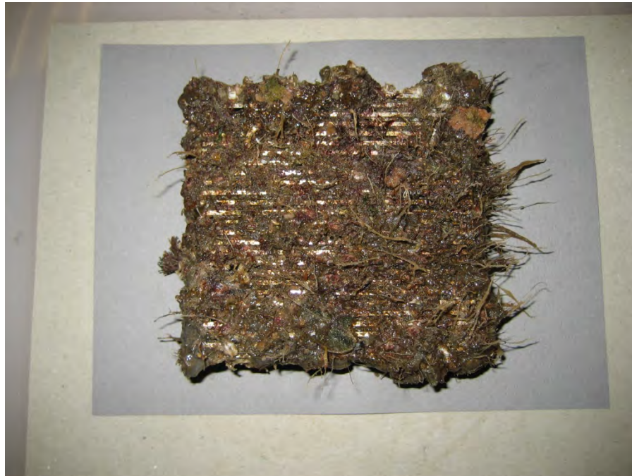
Figure 4-7: 2205 stainless steel Wedgewire sample, photographed 06/17/15.
