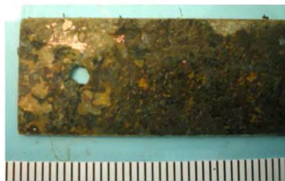
Figure 4-30: Detail view of 90-10 Cu-Ni 1-inch by 3-inch coupon with weld.
