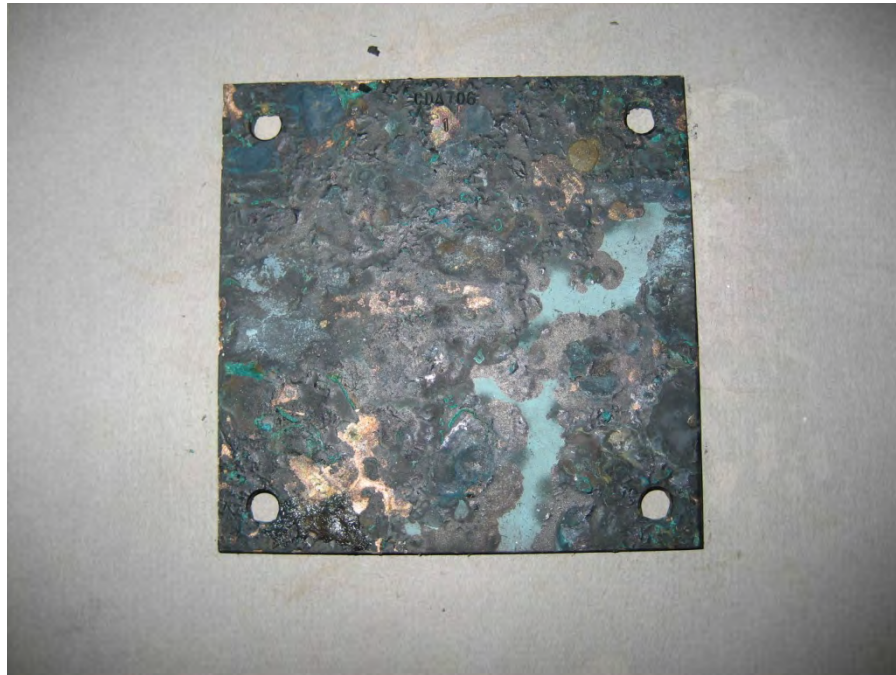
Figure 4-11: 90/10 Cu/Ni (CDA706) test plate (Test Plate 1), photographed 06/18/15 prior to biofouling inspection.
