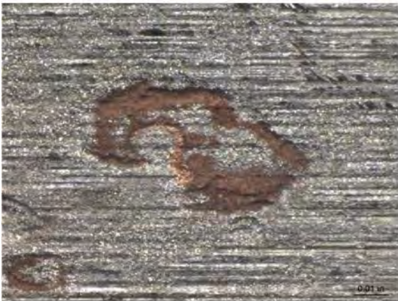
Figure 4-48: CDA 715 coupon at 50X magnification after cleaning.
