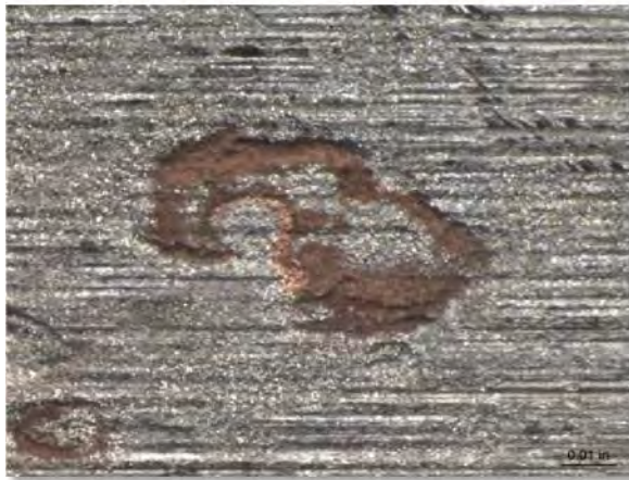
Figure 4-48: CDA 715 coupon at 50X magnification after cleaning.
