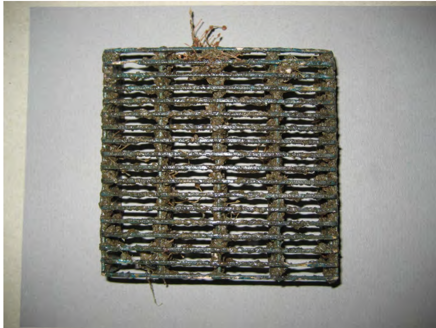
Figure 4-1: 90/10 Cu/Ni (CDA706) Wedgewire sample, photographed 06/17/15.
