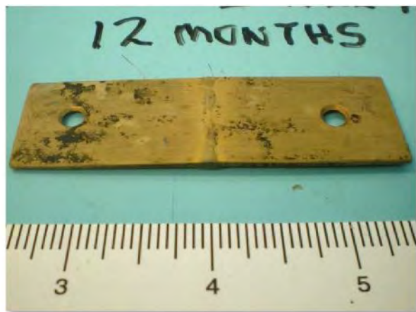
Figure 4-34: Z alloy 1-inch by 3-inch coupon with weld front.
