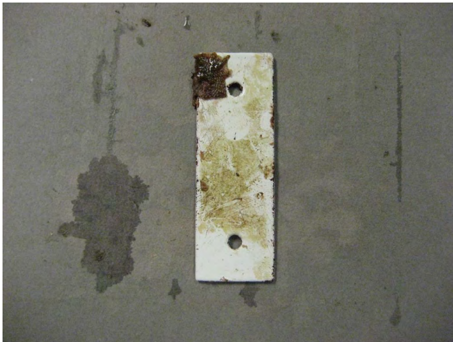
Figure 4-6: 2205 stainless steel coupon with foul release coating, photographed 06/17/15.
