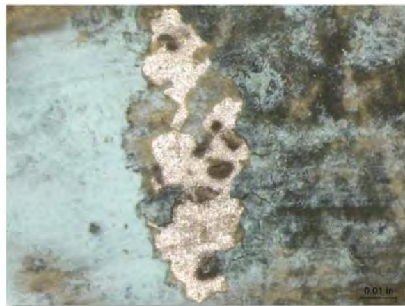
Figure 4-36: Surface discoloration of Z alloy coupon, shown at 50X magnification.
