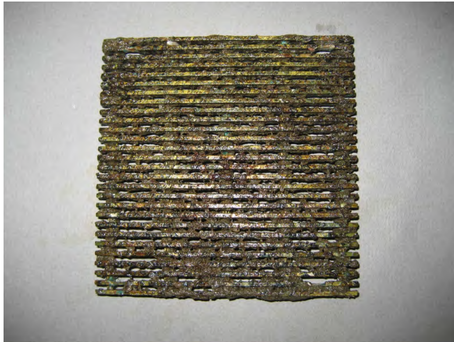
Figure 4-9: 70/30 Cu/Ni (CDA715) Wedgewire sample, photographed 06/17/15.
