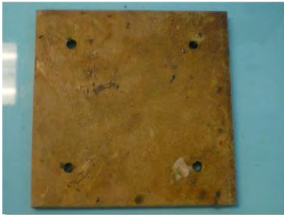
Figure 4-35: Surface discoloration of Z alloy coupon. front (top). back (bottom).
