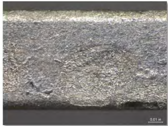
Figure 4-49: CDA 715 screen at 50X magnification after cleaning.
