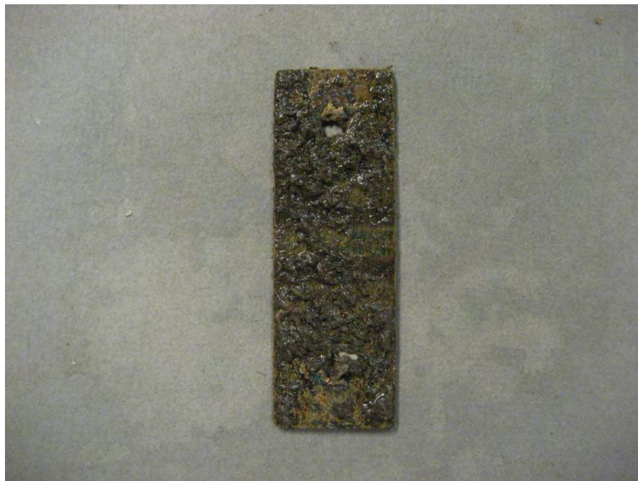
Figure 4-2: 90/10 Cu/Ni (CDA706) coupon, photographed 06/17/15.
