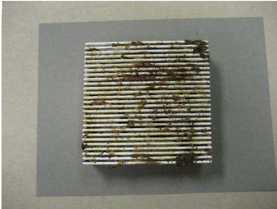
Figure 4-5: 2205 stainless steel Wedgewire sample with foul release coating, photographed 06/17/15.
