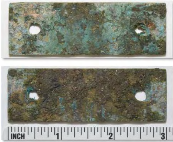
Figure 4-31: Development of patina on 90-10 Cu-Ni coupon, front (top), back (bottom).
