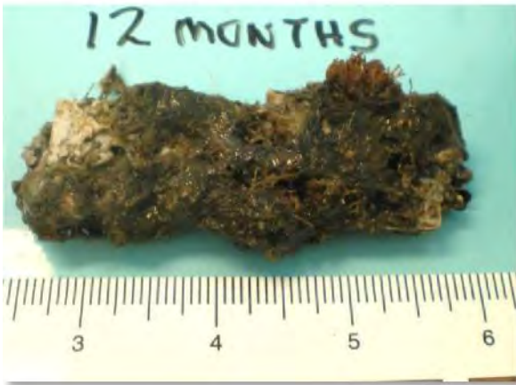
Figure 4-19: Marine life attached to uncoated 2205 Duplex stainless steel coupon with a weld.
