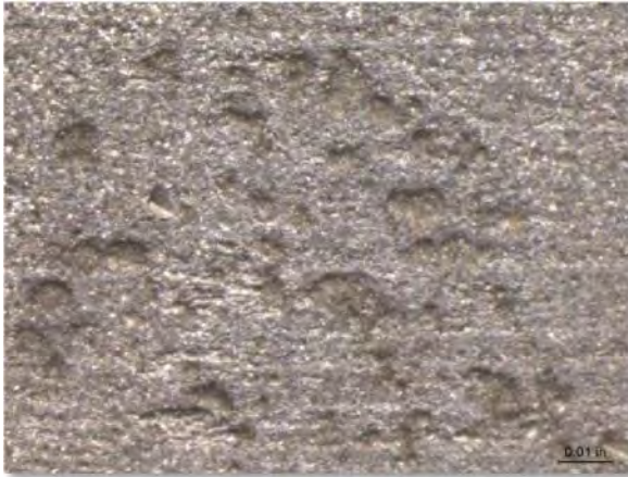
Figure 4-54: Z alloy coupon at 50X magnification after cleaning.
