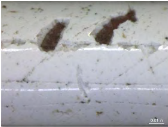
Figure 4-46: 2205 Duplex SS wedge wire screen surface exposed at an area of coating damage. Plate surface after cleaning at 50X
