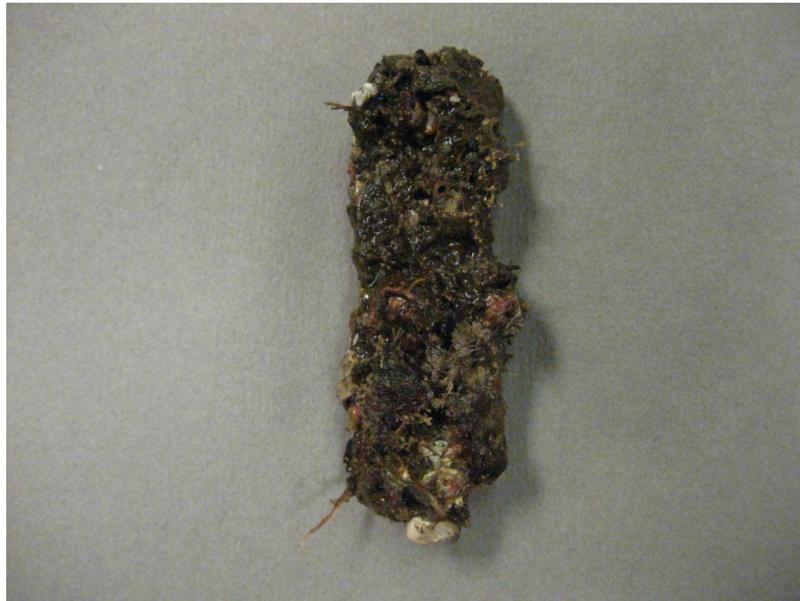
Figure 4-8: 2205 stainless steel coupon, photographed 06/17/15.
