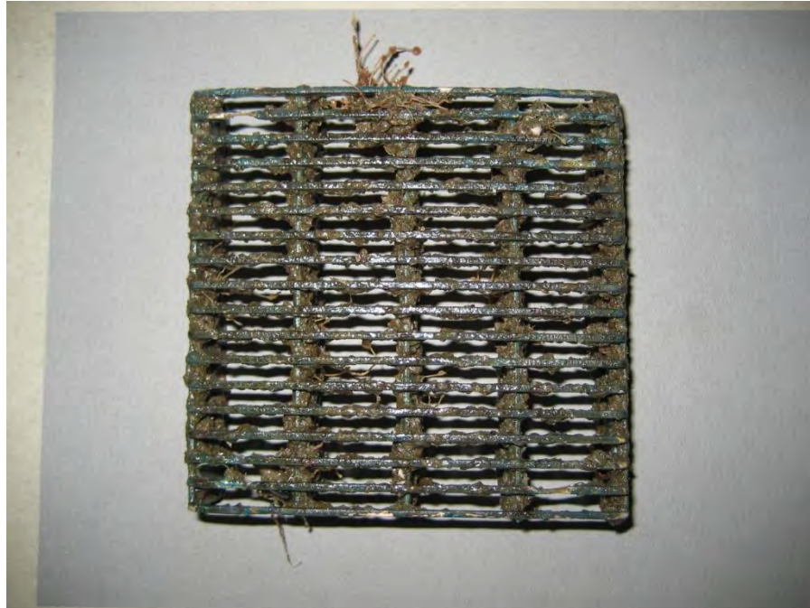
Figure 4-1: 90/10 Cu/Ni (CDA706) Wedgewire sample, photographed 06/17/15.
