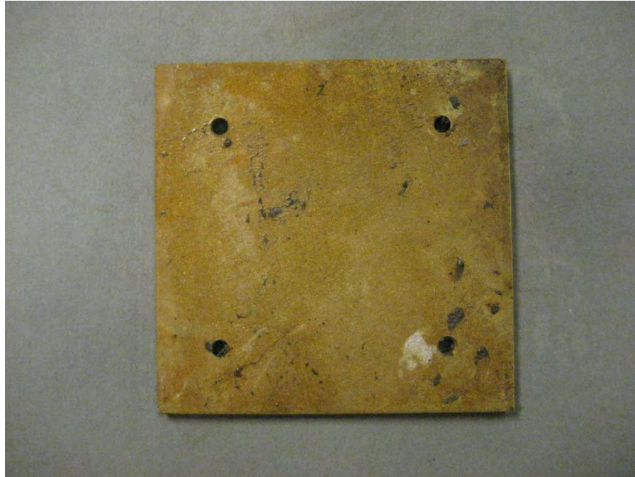
Figure 4-13: Z-alloy test plate (Test Plate 3), photographed 06/18/15 prior to biofouling inspection.
