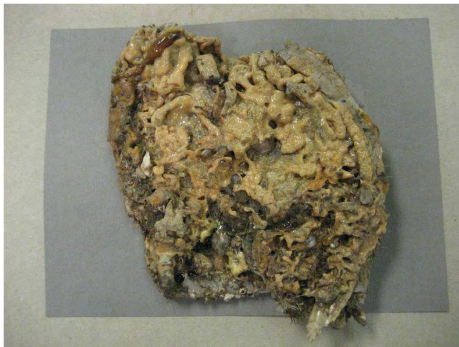
Figure 4-14: 2205 stainless steel test plate (Test Plate 4), photographed 06/18/15 prior to biofouling inspection.
