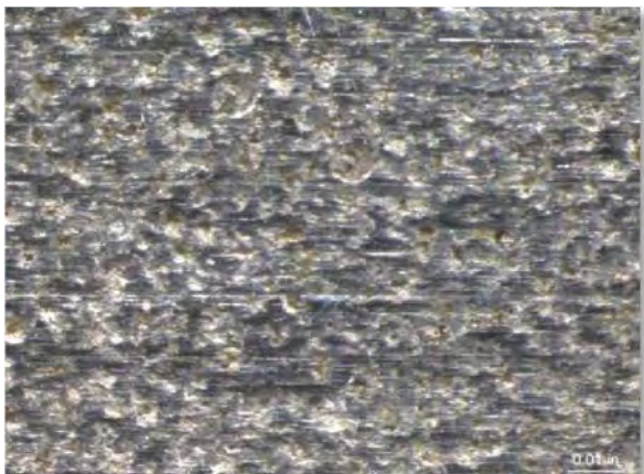
Figure 4-42: Uncoated 2205 Duplex SS coupon surface after cleaning at 50X magnification.
