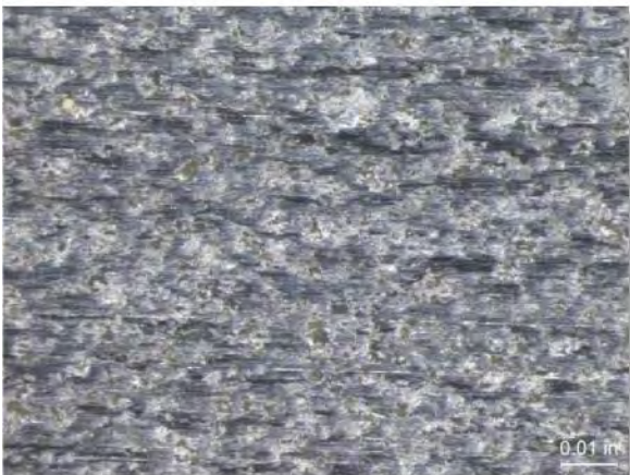
Figure 4-44: Uncoated 2205 Duplex SS plate surface after cleaning at 50X magnification.
