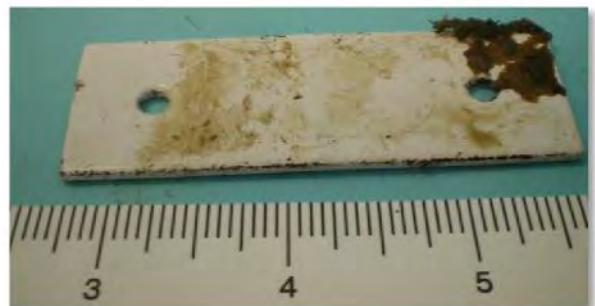
Figure 4-22: Slight damage to coating on edge and initiation of biofouling on corner of coated 2205 Duplex stainless steel coupon.
