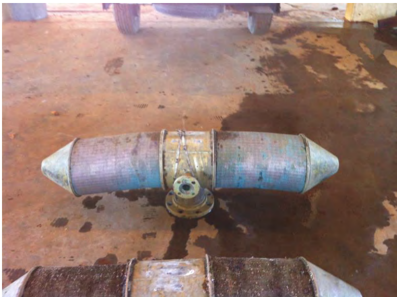
Cook Legacy Screen after Structural Failure
