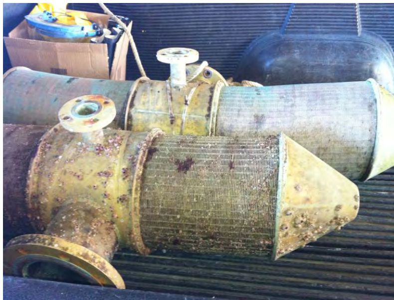
Cook Legacy Screens Removed after Failure
