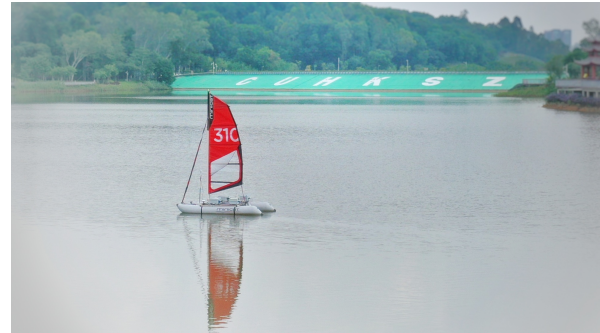
Fig. 1. OceanVoy is sailing in Shenxian Lake, the Chinese University of Hong Kong, Shenzhen. It is equipped with a weather station, RTK-GPS station, power management system, and other devices. Besides, the necessary equipments are installed around the lake, such as the communication station, the weather station and surveillance cameras.
