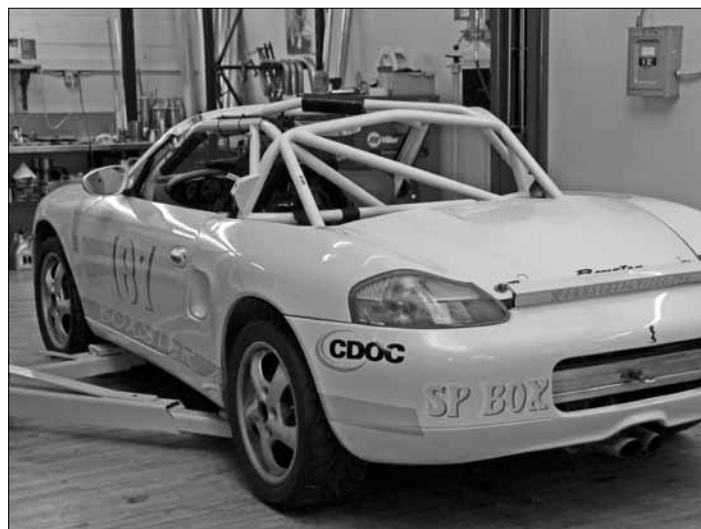
It isn't easy to design a roll cage that fits in a Boxster and is tall enough for Scott Leopold's helmet to satisfy the "broomstick" rule.
