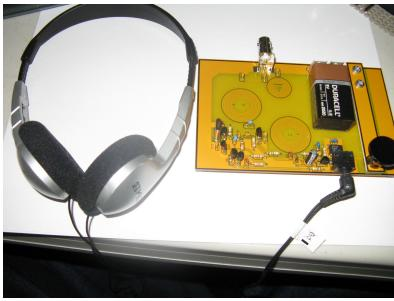
Illustration 5: 500 mw on 80 meters; KT1I's Cricket QRP Transceiver
