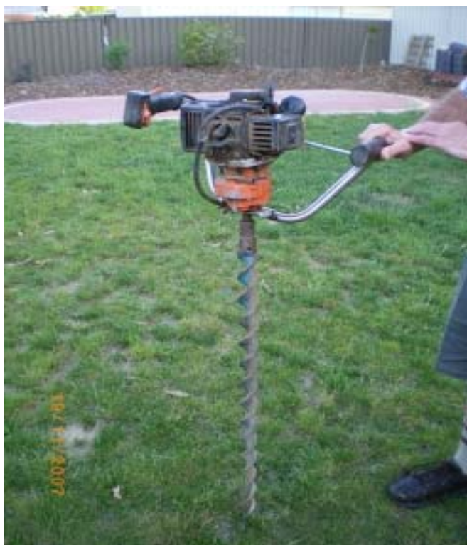
Photograph 1.1: Motorised soil sampler
