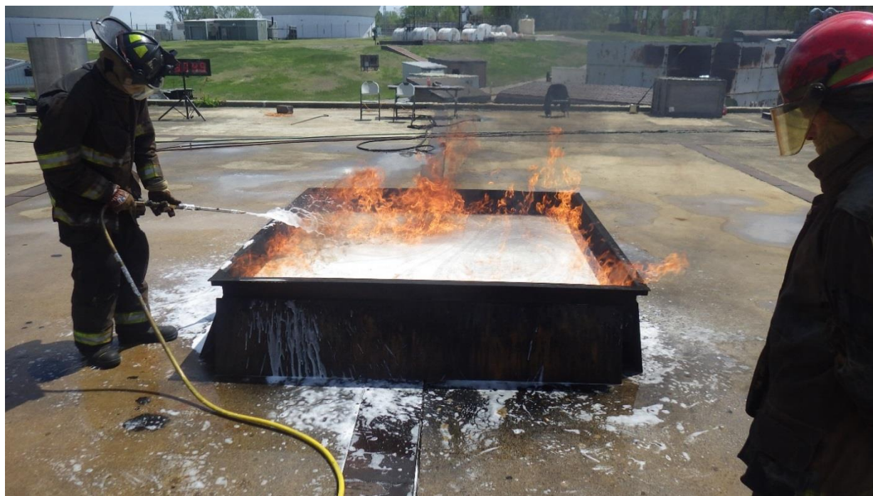
Figure 9.2-3 MILSPEC Gasoline Vapor Penetration of the Lower Aspirated Foam Blanket
