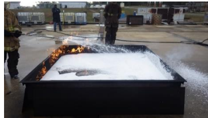
Figure 8.3-1 Direct and Indirect Attacks on Type III IPA Fires
