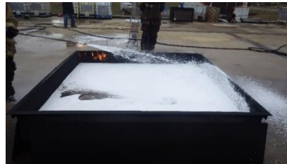
Figure 8.3-1 Direct and Indirect Attacks on Type III IPA Fires
