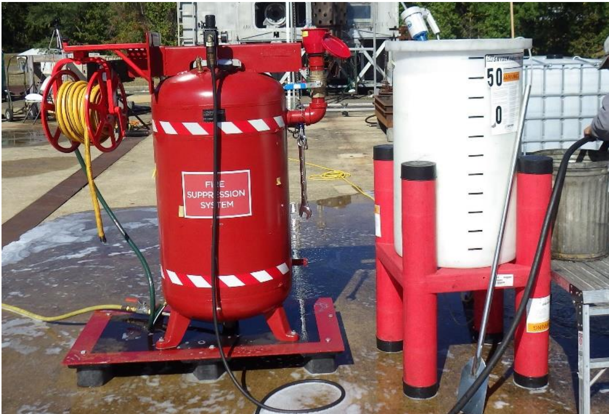
Figure 6.6-1 Foam Mixing and Discharge System
